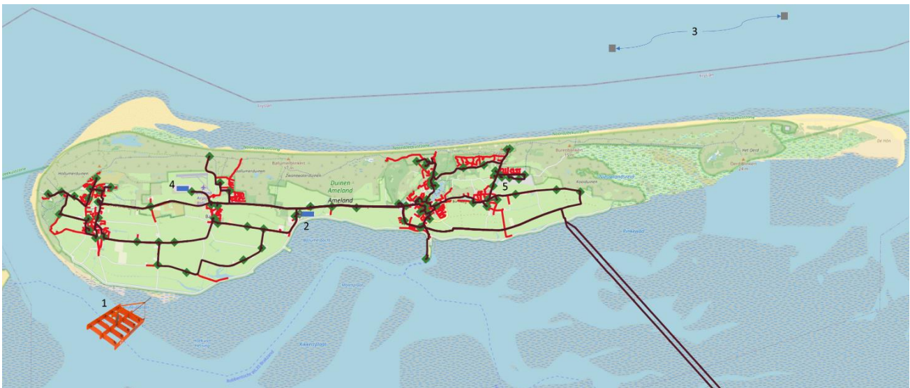
Figure 10 Ameland's grid and assets that are installed or ready to be installed. 1: Tidal Kite, 2: Solar Park Ballumerbocht 3 MW, Battery pack, Electrolyzer, 3: NAM platform, 4: Solar Park Airport 6 MW, 5: Heating Grid Klein Vaarwater, CHP's Klein Vaarwater
