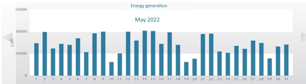
Figure 3: energy production of the 6 MW solar park in May 2022
