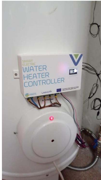
Figure 11: A Smart Electric Water Heater Controller already installed at one household in Terceira Island.
