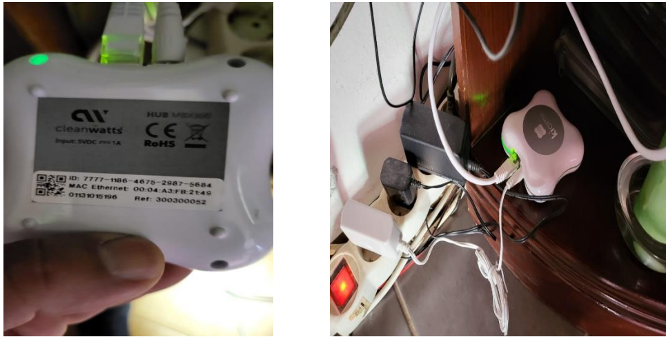
Figure 20: Kiome gateway that has been installed and commissioned.
